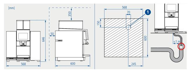
1 Hole diameter 70 mm for water-/milk inlet and water outlet. Also possible for electric cords.
